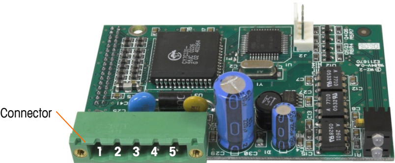
Figure 5-2: DeviceNet Connector Pin Numbering
