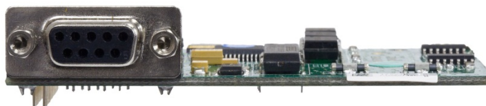
Figure 9-2: PROFIBUS Option Card DB-9 Connector
