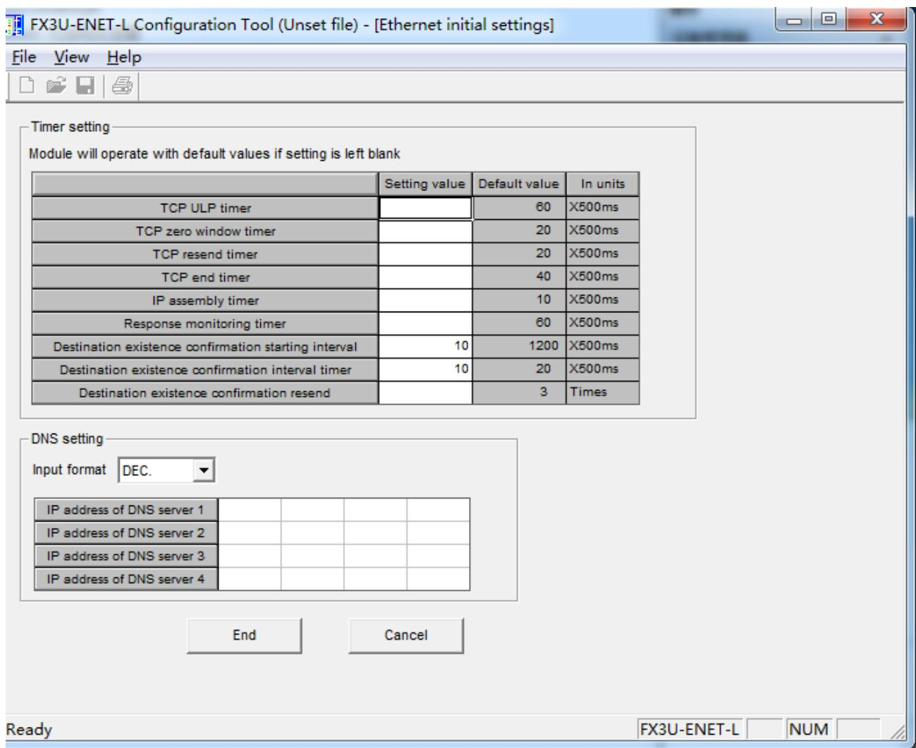
2.1 设置 destination existence confirmation starting interval, destination existence confirmation interval timer, 的Setting value 值10, 设置完成点击End
